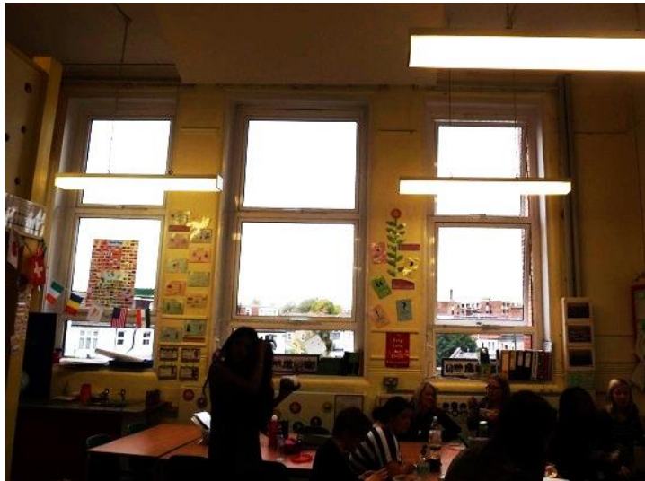
Poor: no external or internal shading control
